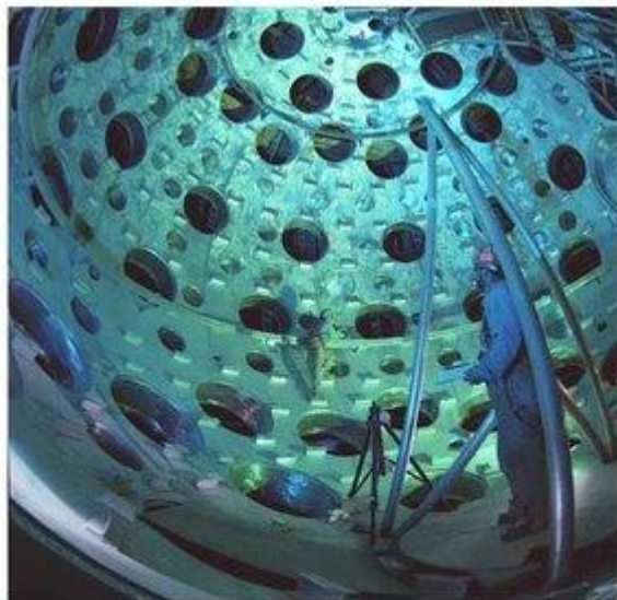
The National Ignition Facility target chamber. 192 laser beams converge on a fusion-fuel-filled target.
