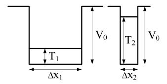
If  $T_{\rm min} = \frac{\hbar^2}{8m\Delta x^2} > V_0$  there is no bound state. We can say that there is no bound state if the potential valley is not enough deep, or the particle is restricted to a very small place. This is the cause that it is impossible for an electron in a nucleus to be in bound state.
