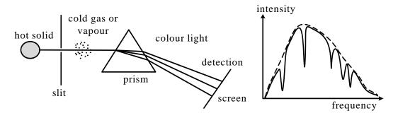
It is a very important fact that a given kind of atom absorbs the same lines when it is cool as it emits when heated. The explanation of the emission and absorption spectra is that the energy of the lonely atom or molecule could be only discrete value. Bohr explained the atomic spectra in 1913.
