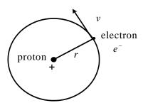
The negatively charged electron of the hydrogen atom is forced to a circular motion by the attractive electrostatic Coulomb force of the positively charged atomic nucleus at rest. The equation of motion:
