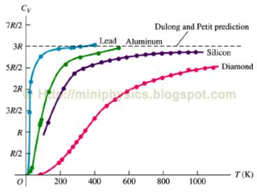
Einstein was who solved the problem with the help of the quantum hypothesis. He supposed that the Planck quantum hypothesis can be applied not only to the energy of the electromagnetic field, but for the energy of the crystal oscillator as well. By employing Planck's quantization assumption, Einstein's theory was in good agreement with observed experimental results.
