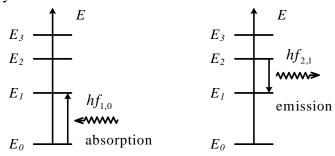
For example the absorbed frequency:  $f_{1,0} = \frac{E_1 - E_0}{h}$ , and the emitted frequency
