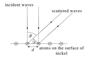
They found a periodical variation of the reflected electron beam intensity due to interference, and the obtained wavelength was in good agreement with the de-Broglie hypothesis. The condition of maximal intensity in case of interference is the path difference is  $d \sin \theta = n \cdot \lambda$ , if n=1,  $d \sin \theta = \lambda$ .
