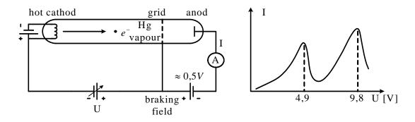
First the electrons are accelerated and collide with mercury atoms but the collision is elastic.
