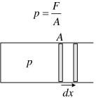
If one wall of the container is moveable the force exerted by the gas may produce a displacement dx of the wall. Therefore the elementary work done by the gas:
