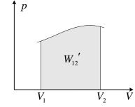
The geometrical meaning of the integral is the area under the curve. So the work done by the system in going from  $V_1$  to  $V_2$ :
