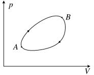
We can approximate the actual cycle by connecting the isotherms by suitably chosen adiabatic lines, thus forming an assembly of Carnot cycles. The adjacent Carnot cycles have a common isotherm and the two travels; in opposite directions cancel each other in the region of overlap as far as heat transfer and work done are concerned. We can write then, for the isothermal-adiabatic sequence of lines as:
