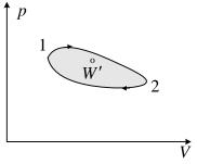
When a system is carried through a cyclic process its initial and final internal energies are equal. So the total internal-energy change in any cyclic process is zero. Apply the first law for a cyclic process:
