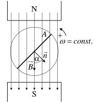
At t = 0 be  $\vec{n} \uparrow \uparrow \vec{B}$ , where  $\vec{n}$  is the normal of the coil. As  $\omega = \text{const.}$ , the angle  $\alpha = \omega t$ . The flux through each turn is  $\Phi = BA \cos \alpha = BA \cos \omega t$ .
