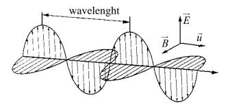
This is a "snapshot" representation of the travelling electromagnetic wave showing the alternating electric and magnetic vectors along the propagation.
