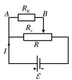
In case of loaded divider the potential difference is not a linear function of the  $R_x$  resistance.
