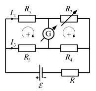
This arrangement of resistors is called Weatstone bridge.  $R_x$  is the unknown resistance. One resistor is varied until the current in the galvanometer G is zero. The bridge is then said to be balanced.  $I_G = 0$
