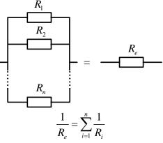
For any number of resistors in parallel, the reciprocal of the equivalent resistance equals the sum of the reciprocals of their individual resistances.
