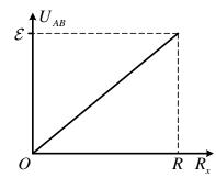
The potential divider is loaded if the variable potential difference is applied on a consumer  $R_{\kappa}$ .
