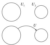
If we connect the two conductors with a conductor wire, then charge flows through the wire until the potential of the united conductor equalize. The charge transfer directed from the higher potential to the lower one.
