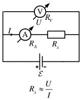
In case of digital multimeters an operational amplifier is used to increase the internal resistance of the voltmeter to  $\sim 10 M\Omega$ . This resistance is so large that does not disturb the circuit. The current measurement is really a potential difference measurement on a high accuracy resistor.
