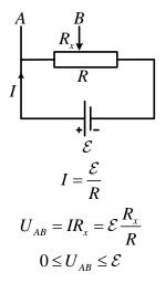
The value of  $U_{AB}$  can be varied by moving the sliding contact of the resistor. This voltage is linear function of  $R_x$ .
