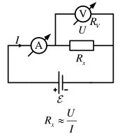
b) if  $R_x >> R_A$  (internal resistance of ammeter)
