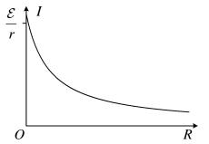
If the terminals of a source are connected by a conductor of zero (or negligible) resistance, the source is said to be short circuited. The short-circuit current is:
