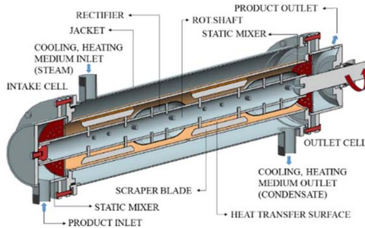
Fig. 1. Vertical cross section at center line through the horizontal SSHE,  $D_{jacket-in}=172$  mm,  $D_{heat-transfer-in}=98.8/122.9$  mm,  $d_{shaft-out}=48/60$  mm
