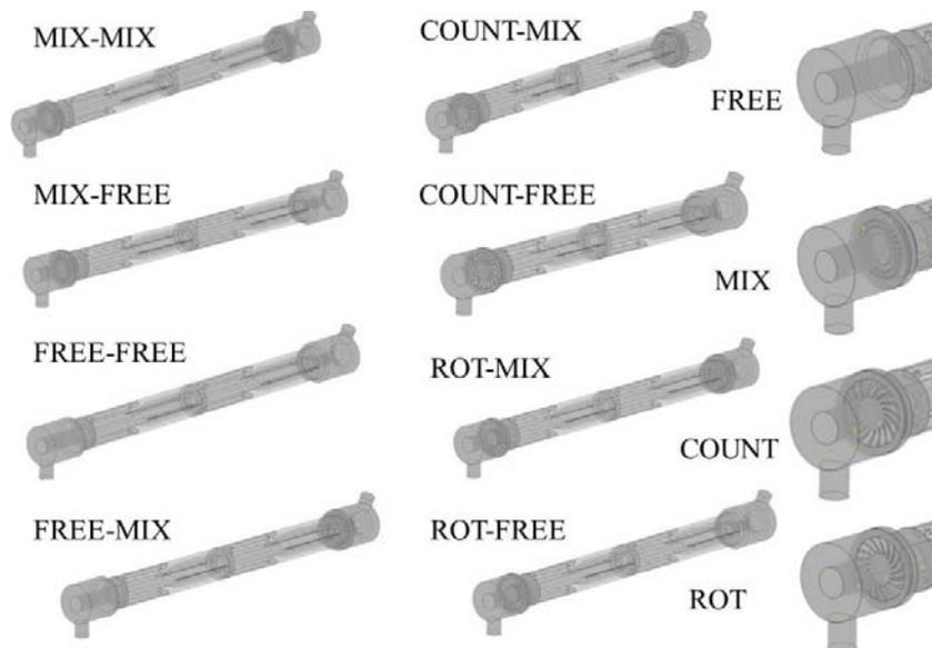
Fig. 2. variations of used static mixers and their positions for numerical analysis
