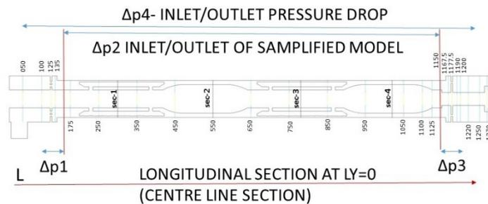
Fig. 3.  $\Delta p1-4$  checked pressure drops between positions as marked
