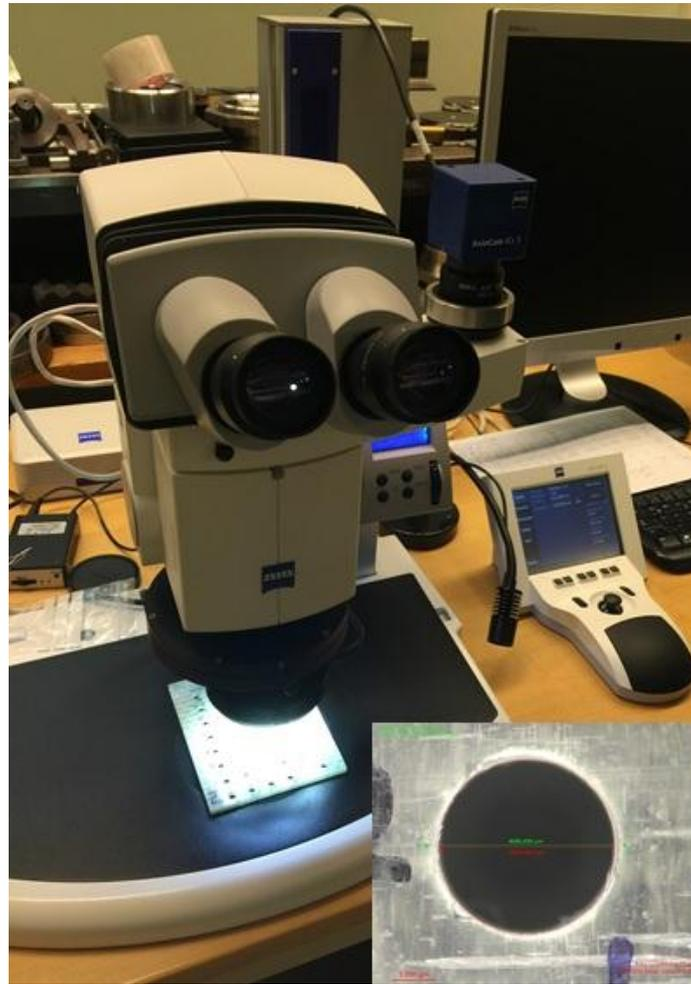
Figure 1: The delamination measurement view using optical stereomicroscopy [16]
