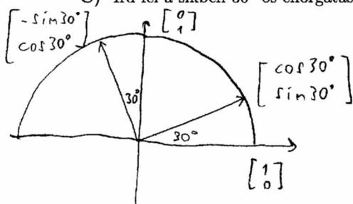
$$R_{30^\circ} = \begin{bmatrix} \cos 30^\circ & -\sin 30^\circ \\ \sin 30^\circ & \cos 30^\circ \end{bmatrix} = \begin{bmatrix} \sqrt{3}/2 & -1/2 \\ 1/2 & \sqrt{3}/2 \end{bmatrix}$$
