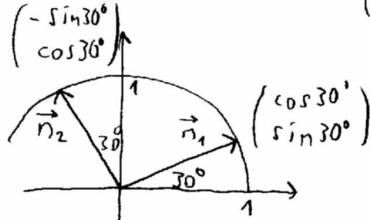
$$y_1 = (\vec{n}_1, \vec{x}) = \left( \begin{pmatrix} \cos 30^\circ \\ \sin 30^\circ \end{pmatrix}, \begin{pmatrix} 3 \\ 4 \end{pmatrix} \right) = (\cos 30^\circ, \sin 30^\circ) \begin{pmatrix} 3 \\ 4 \end{pmatrix}$$
