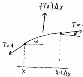
$$\begin{aligned} \sin \alpha &\approx \tan \alpha = \varphi'(x) \\ \sin \beta &\approx \tan \beta = \varphi'(x + \Delta x) \\ &\approx \varphi'(x) + \varphi''(x) \Delta x \end{aligned}$$
