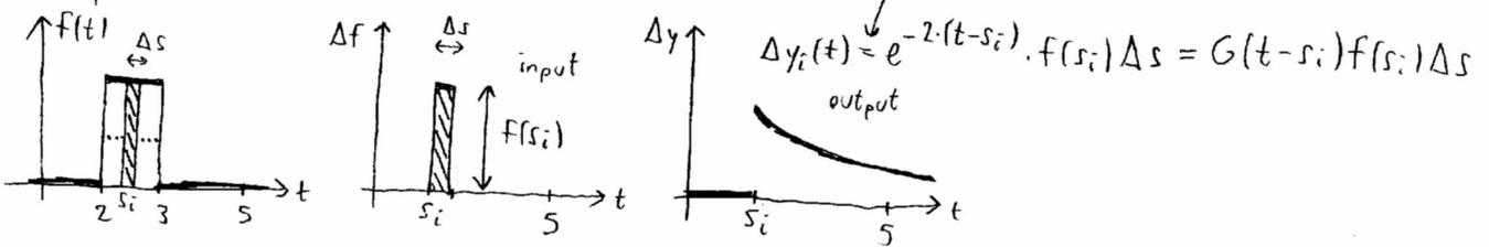
$$y(t) = \sum_i \Delta y_i(t) = \sum_i e^{-2(t-s_i)} f(s_i) \Delta s = \int_0^t e^{-2(t-s)} f(s) ds = \int_{-\infty}^{\infty} G(t-s) f(s) ds$$
