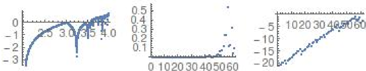
Figure 2.20: a) Lyapunov exponent of the logistic map f(x) = rx(1 - x) as a function of r . It is measured as the average of \ln(|f'(x_n)|) for n = 100, \dots, 250 . b) |x_n - \tilde{x}_n| , where r = 3.7 , x_0 = 0.3 , \tilde{x}_0 = x_0 + 10^{-9} . c) \ln(|x_n - \tilde{x}_n|) . We can estimate the Lyapunov exponent as the slope of a straight line approximation of this plot in a region where |x_n - \tilde{x}_n| is small. The slope in the n = 10, \dots, 30 region is 0.352. Compare this to the more precise value \lambda = 0.3704 from the first plot.
