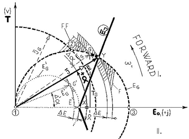
Fig.2. Induction machine combined Contact Energy and Contact Energy Control diagram
