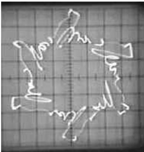
Fig. 11. Voltage space vector trajectory
