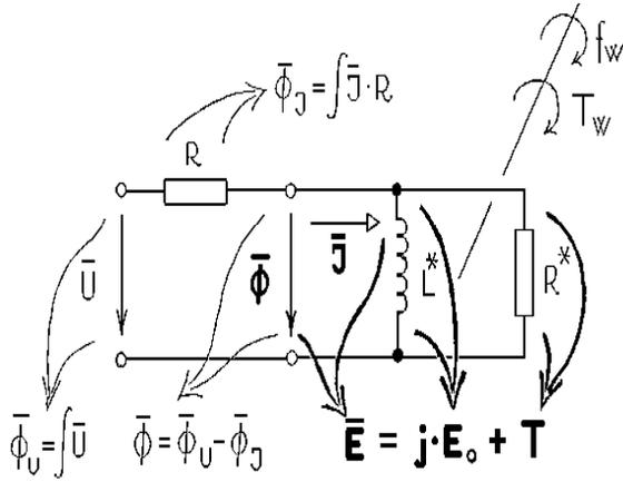
Fig. 3. Induction motor contact energy model
