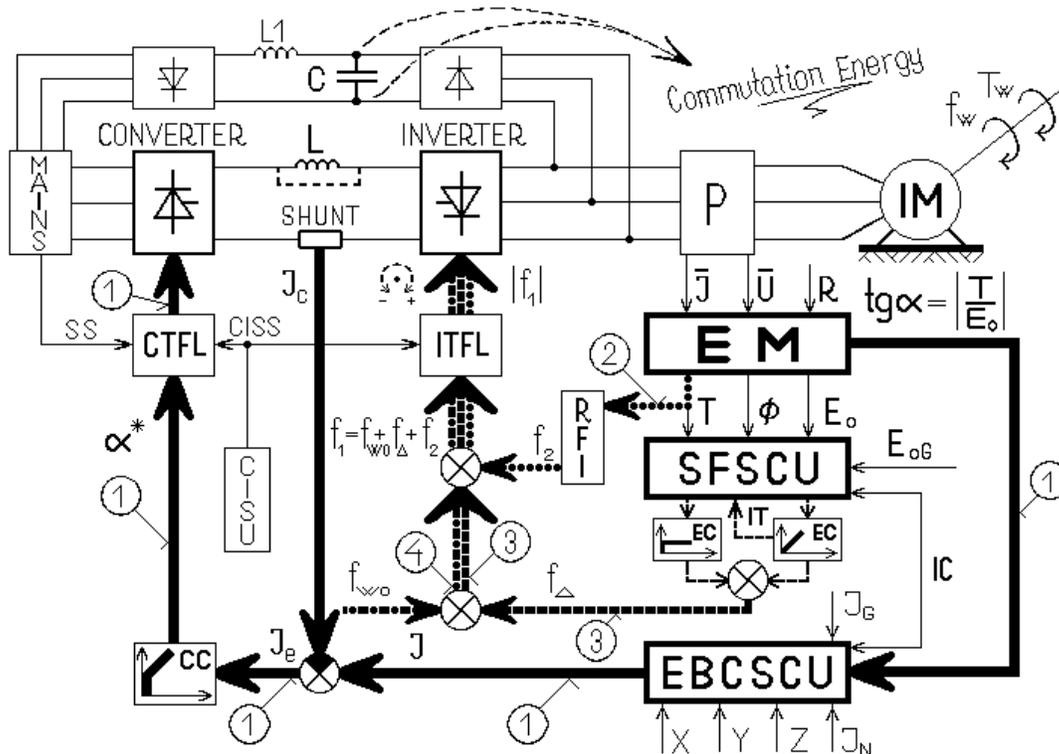
Fig. 1: Energy Based Current Control (EBCC)
