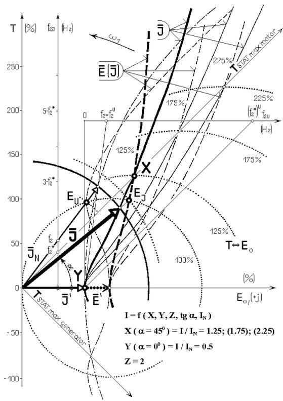
Fig. 5. Energy Based Current Control diagram of induction machine
