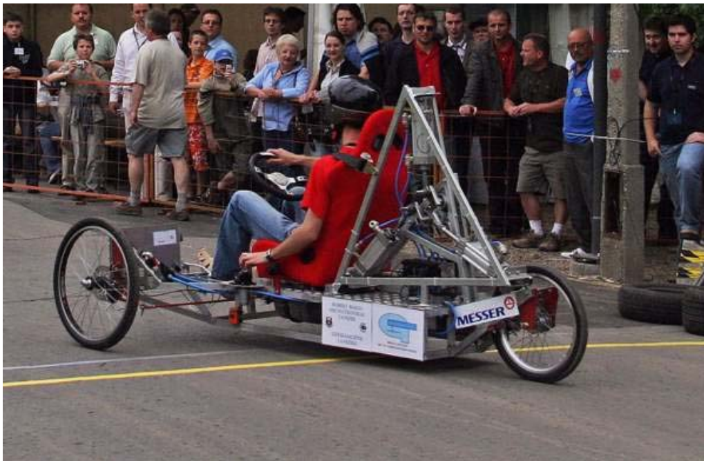
Figure 3. The modified Pneumobile
