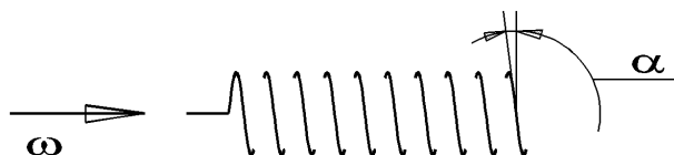
Figure 8. The hollow cylinder having large split angle is a helical spring
