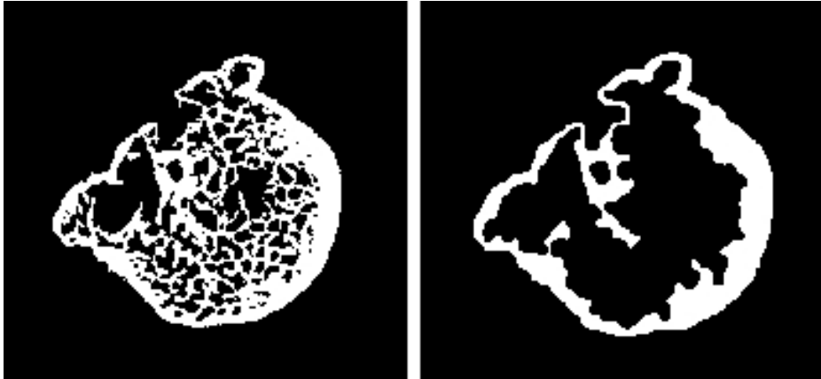
Figure 3. The image right after binarization (left), the image after elimination the small object (right)
