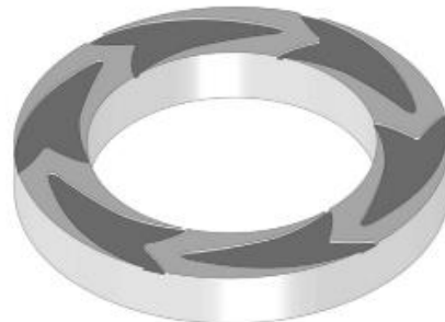
Figure 2. Standing pad of hydrostatic thrust bearing allocated with optimized grooves
