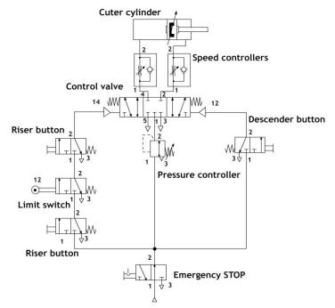
Figure 1. The pneumatic circuit in progress
