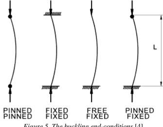
Figure 5. The buckling end-conditions [4]
