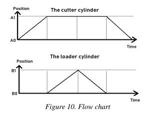
The loader cylinder can pushes the cheese on the cutter surface, or pushes out the pieces of the cut cheeses, above the blade to a conveyor belt.
