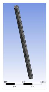
Figure 7. The rod after meshing
