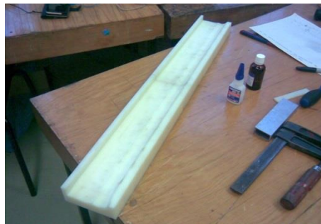
Figure 16. The glued polishing trough
