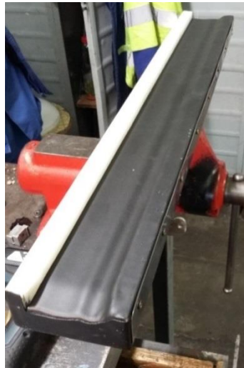
Figure 3. Polishing trough for a 9 grams hollow figure
