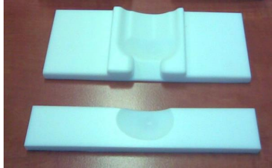
Figure 2. Lifting/pushing tools for 17.5 grams chocolate hollow figures
