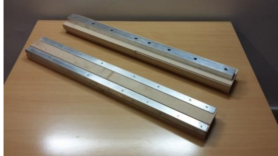
Figure 18. The bottom view of the ready polishing trough and pressing tool. Aluminium strengthening can be seen here
