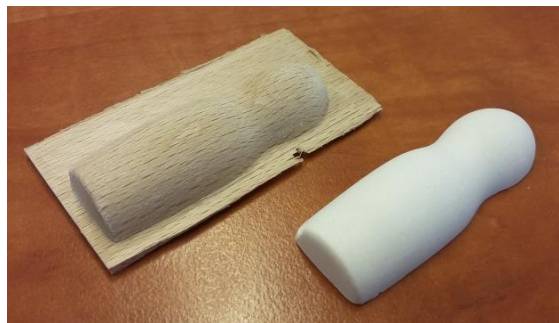
Figure 6. The manufactured sample with Roland MDX650A (left) and the original gypsum sample (right)
