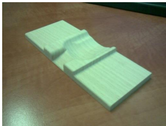
Figure 19. Lifting tool made of steamed beech
