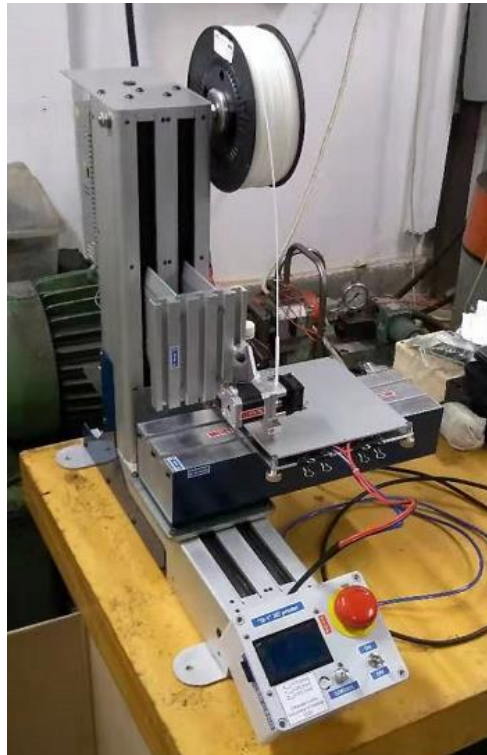
Figure 3 The assembled 3D desktop printer
