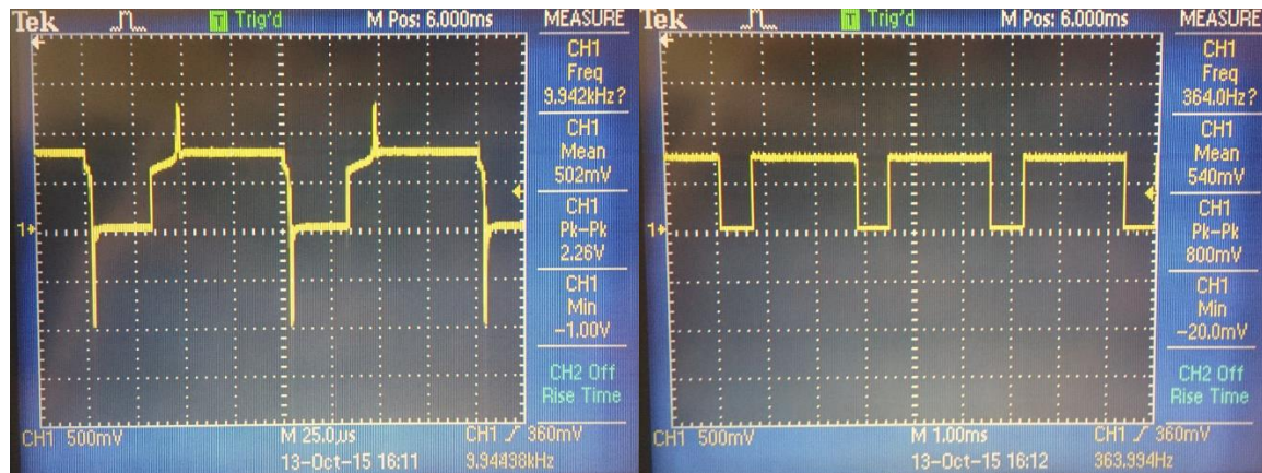
Figure 8 Control signals of the higher frequency output (left), and lower frequency output (right)
