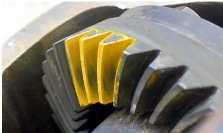
Figure 2. The formed contact pattern on the tooth surface (the worn area) [10]
