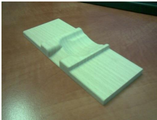
Figure 19. Lifting tool made of steamed beech
