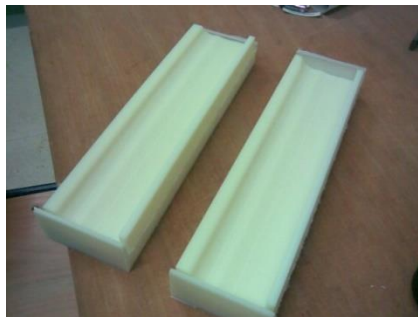
Figure 12. Parts of the packaging tool made from PA6
