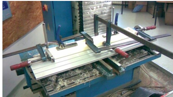
Figure 15. Pressing the parts of the trough
