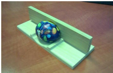
Figure 21. Pushing and lifting tools made of steamed beech and the packed chocolate egg
