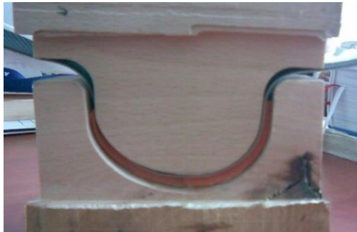
Figure 11. Gluing and pressing of the short version of the trough (for 17,5 g chocolate egg)
