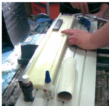
Figure 14. Gluing the parts of the polishing trough
