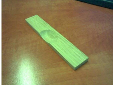
Figure 20. Pushing tool made of steamed beech
