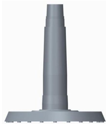
Figure 3. The 3D CAD model of the spindle – milling-disk assembly
