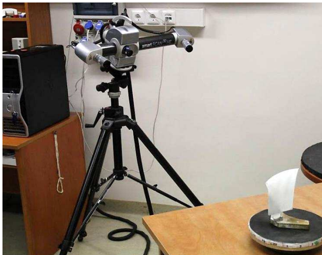
16. ábra BREUCKMANN SMART SCAN 3D-HE optikai szkennert a Reverse-Engineering Laborban
