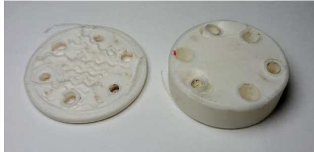
Figure 8. Failed part of the gearbox – output flange
