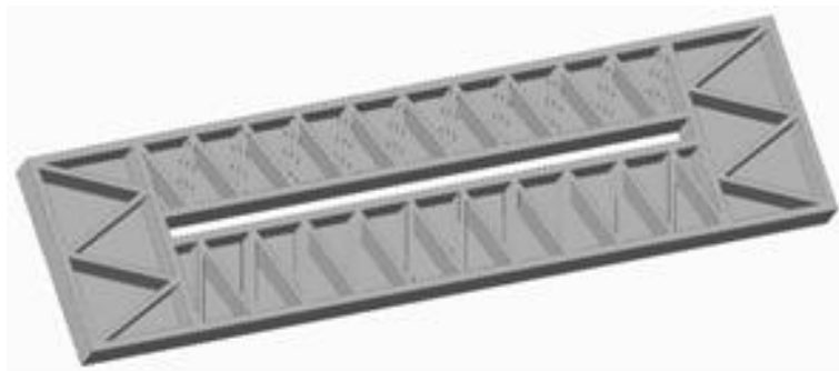
Figure 1. Ribbed structure with aluminium material
