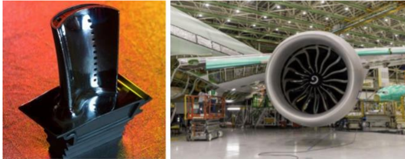
Figure 1. 3D printed Ti-Al alloy blades for Boeing power units [5]
