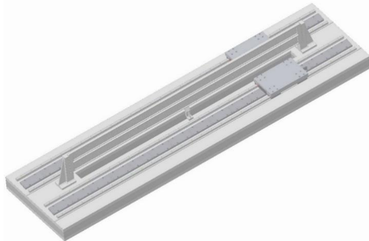
Figure 2. Table with composite structure equipped with guideways
